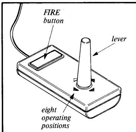
Each handheld unit has two operating controls, the lever and the FIRE button. The four marks around the base of each lever indicate the eight main lever positions available in addition to the centre position and the four diagonal positions.
