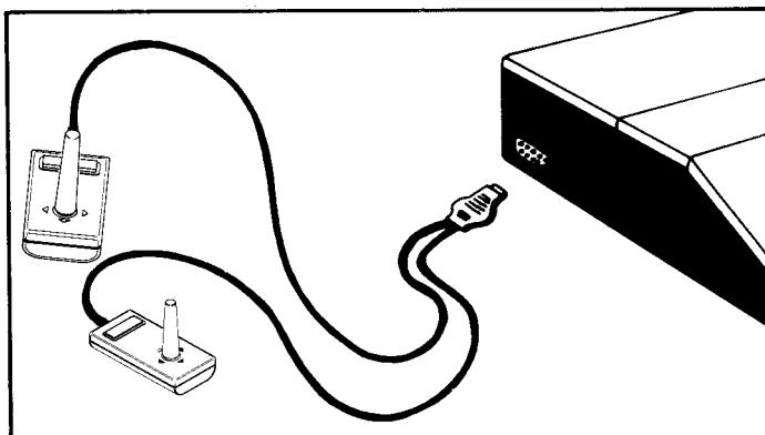
The cable can be plugged in at any time without disturbing the module activity or TI BASIC program in progress. Some applications require both handheld units, while other activities use only one.
