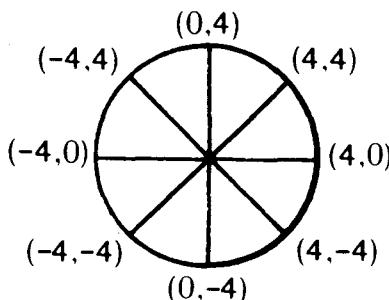
When the CALL JOYST statement is performed, integer values of -4, +4, or 0 are automatically assigned to the *X*- and *Y-returns*, based on the position of the lever.
