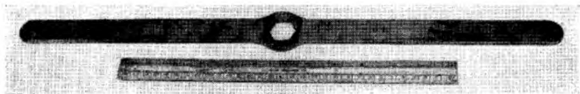
Fig. 10. SPANNERS, sparking plug, \frac{1}{2} in. Whitworth. Ref. No. 4N/9.
