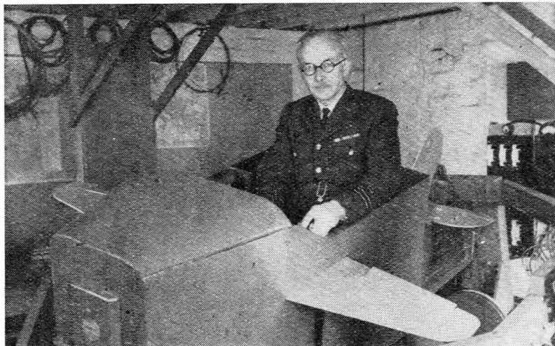
A view of the trainer which shows the supporting frame on the left. Notice the ailerons and roomy cockpit. Seated at the controls is Flight Lieutenant Whittington, the Commanding Officer.
