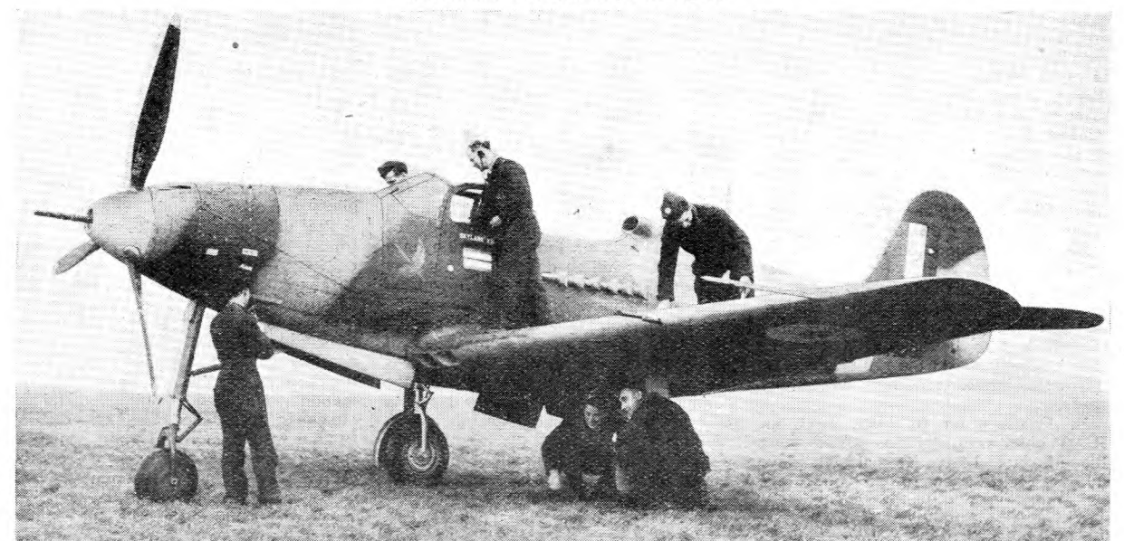
Maintenance on an Airacobra in operation with Fighter Command. The exhaust pipes and air intake visible behind the cockpit give indication of the rearward-placed engine.
