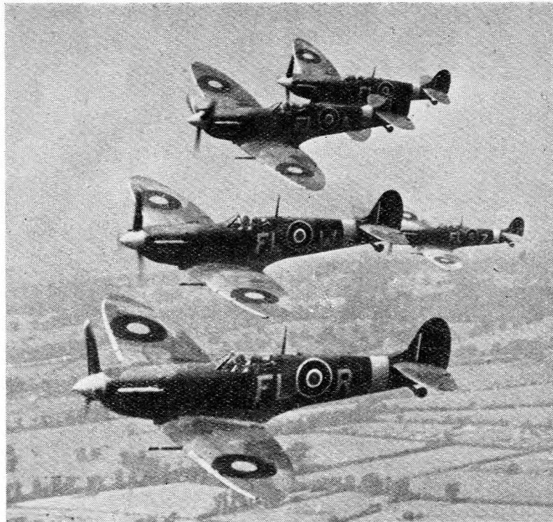
Supermarine Spitfire VB twin-cannon fighters of the R.A.F., whose engine, the Merlin XLV, is quoted as having a maximum power of 1,300 h.p., giving a top speed in the region of 370 m.p.h.
