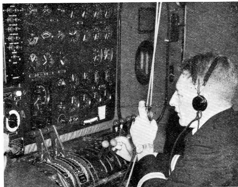
A Flight Engineer at the control panel of the Boeing Bristol. The two nearest levers operate the engine cowl flaps.
