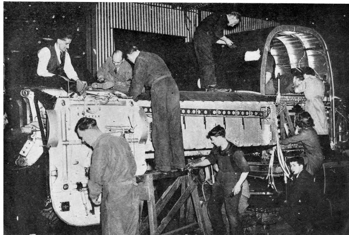
Men and women at work on the centre section of a Halifax
