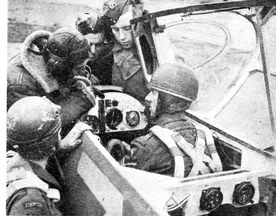
Gliding instruction for prospective Army pilots. Note the crash helmets and that the glider, a General Aircraft Hotspur II, is apparently equipped with a second cockpit for dual instruction. Army glider pilots first train on powered aircraft and then on dual control gliders.
