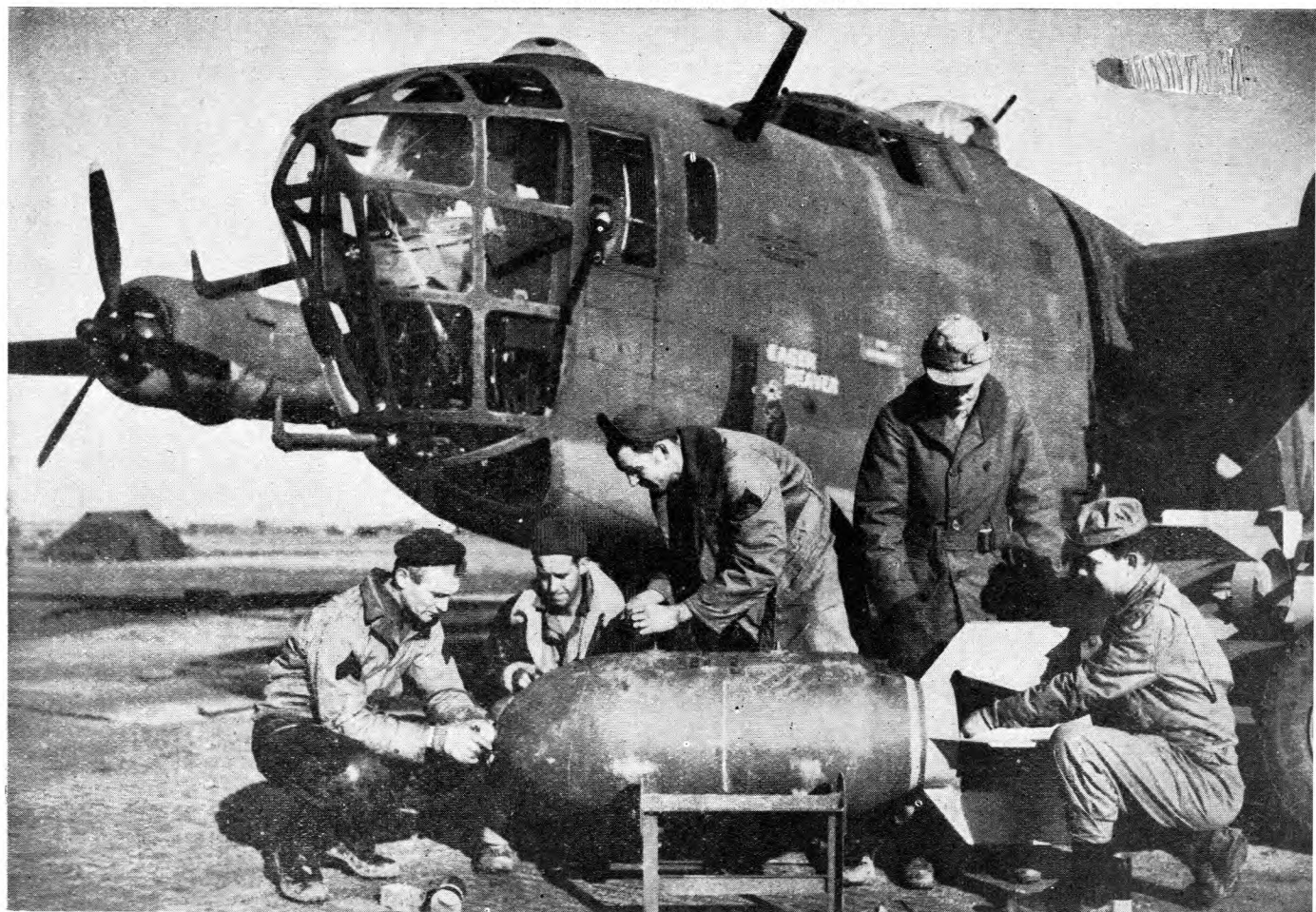
Men of the U.S. Army Eighth Air Force priming and "finning" American-built 1,000-lb. bombs before loading them into a Consolidated B-24 heavy bomber (span 110 ft.).
