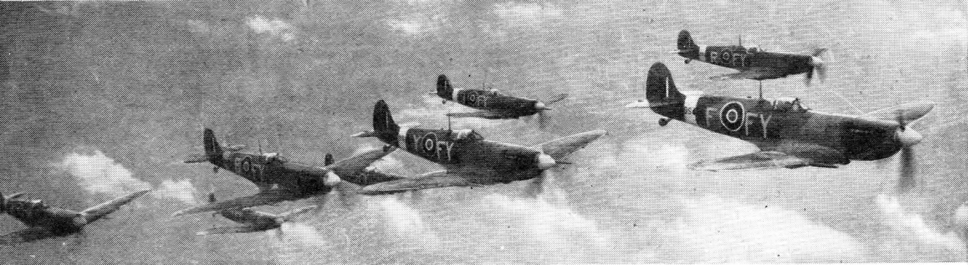
A formation of Supermarine Spitfire IXs above the clouds. This version of the Spitfire is fitted with the Rolls-Royce Merlin 61 engine and has a four-bladed airscrew. No dimensions may be published.
