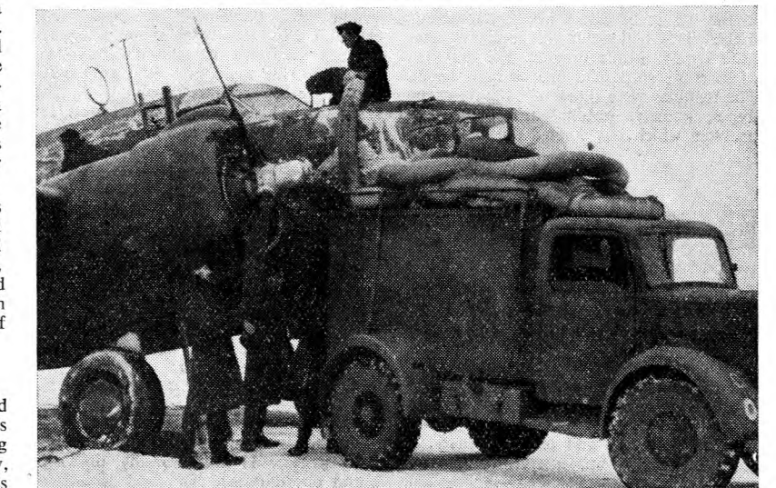
Engines are warm-blooded things. This hot-air van is used to de-ice a Hudson of Coastal Command operating in wintry weather.
