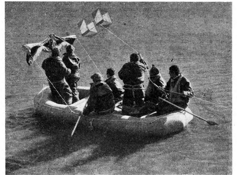
Launching a kite to carry the radio aerial of an American dinghy.
