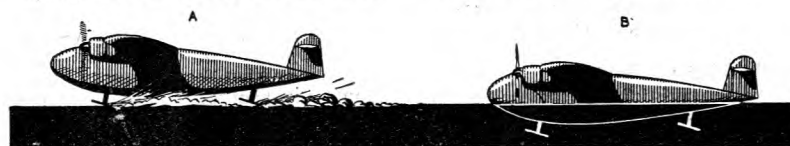
Hydrofoils: (a) hydroplaning, (b) at rest.
