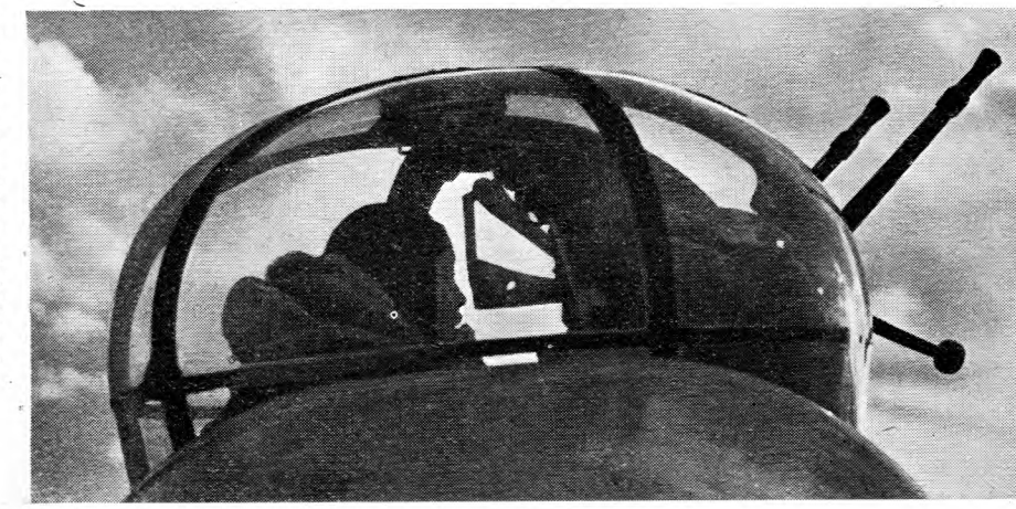
The mid upper gun turret of a Lancaster. It is a Frazer-Nash 50 with two .303 calibre Browning machine-guns. Below the gun can be seen an "interrupter" which prevents the gunner from hitting his own tail.
