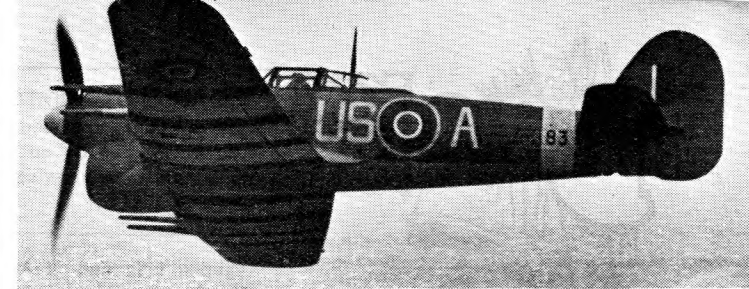
The Typhoon Ib. The zebra-like markings on the underside of the wings are to avoid confusion with the Focke-Wulf 190.
