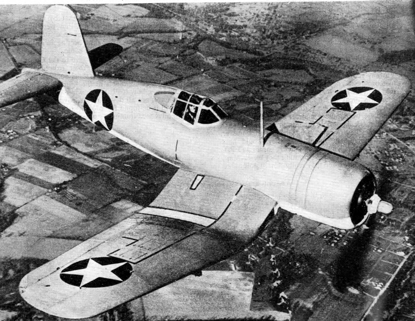
The Vought-Sikorsky Corsair, America's newest naval fighter. Powered by a Pratt and Whitney Wasp 2,000 h.p. engine, it has a maximum speed of over 400 m.p.h. Armament consists of three .5 Browning machine-guns in each wing.
