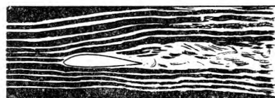
Early separation of airflow at small angle of attack at low Reynolds Number.
