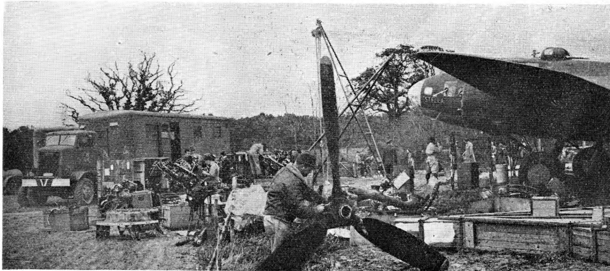
The mobile repair unit here pictured at work has saved the U.S.A.A.F. thousands of dollars and months of labour. This crashed Fortress on which the men of the mobile repair depot are at work made a forced landing somewhere on the South Coast. A special runway was laid down by an engineer unit of the U.S. Army and the Fortress was flown back to her station.
