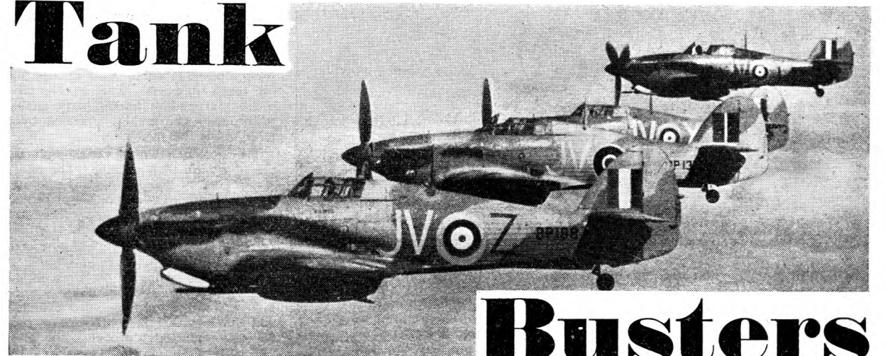
Hawker Hurricane II-Ds in formation. These are armed with two 40-mm. cannon and two .303 machine-guns.
