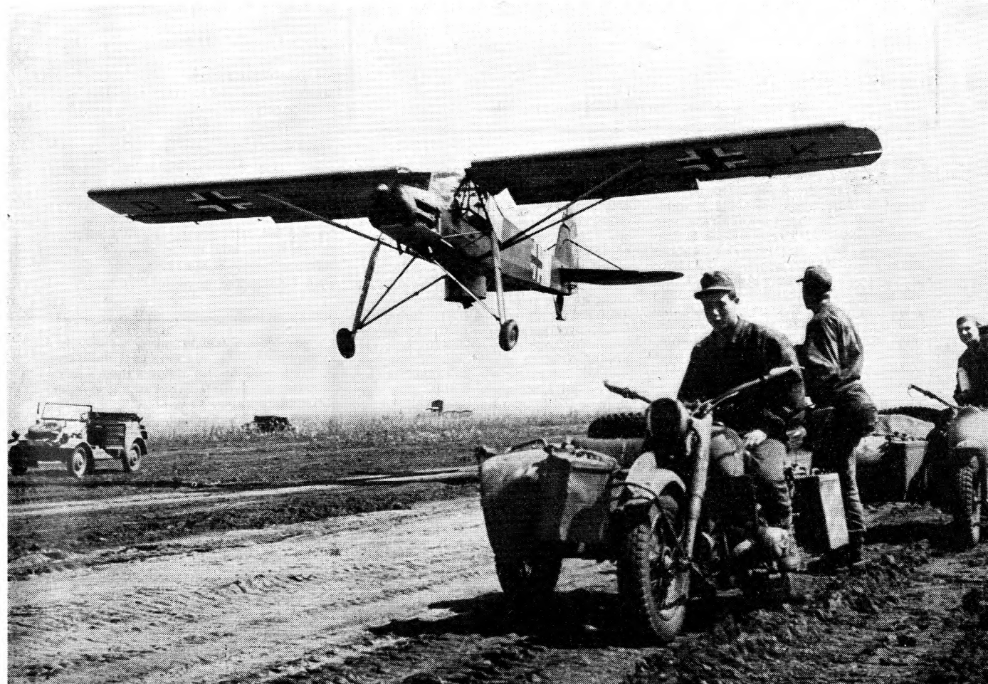
Below: A not-so-new German aircraft, the Fieseler 156 Storch, about to land on a road in Russia. This aircraft has a top speed of 109 m.p.h., landing speed of 31 m.p.h., take-off run of 71 yards and a landing run of 27 yards.
