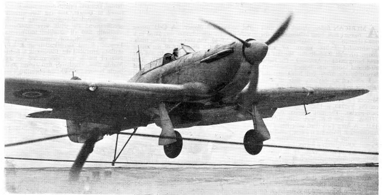
A Sea Hurricane lands on the deck of H.M. Aircraft Carrier Argus. This aircraft's covering is partly stressed and partly fabric.
