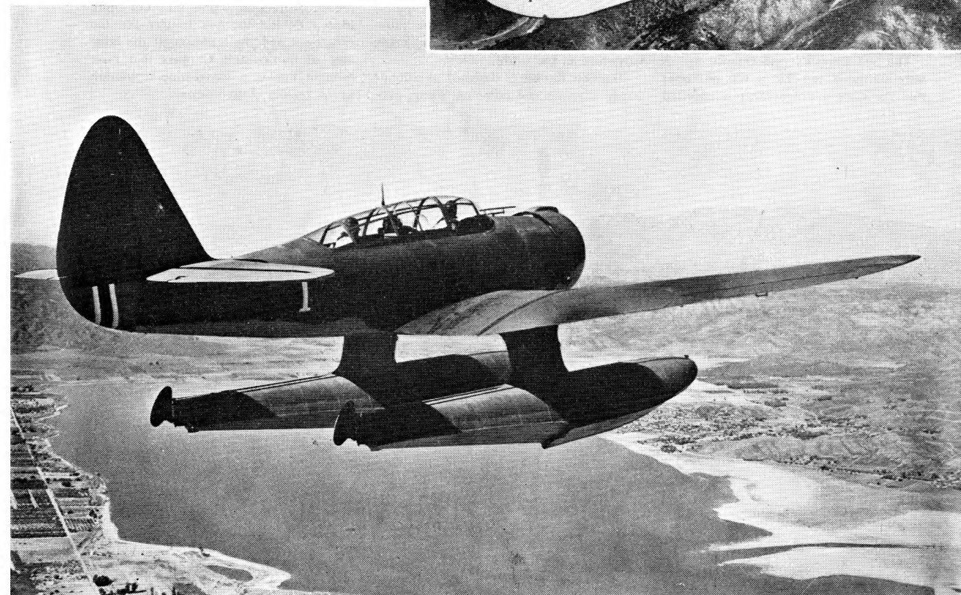
Below: The Northrop N-3PB U.S. Patrol Bomber seaplane. This aircraft is designed for operation against surface craft, and is said to be the fastest float seaplane in the world. It carries a crew of three, has four fixed .5 calibre machine-guns in the wings and one .5 covering the rear, and one .3 firing aft out of the bottom of the fuselage. Maximum speed is 257 m.p.h. Maximum range 1,200 miles at 172 m.p.h.
