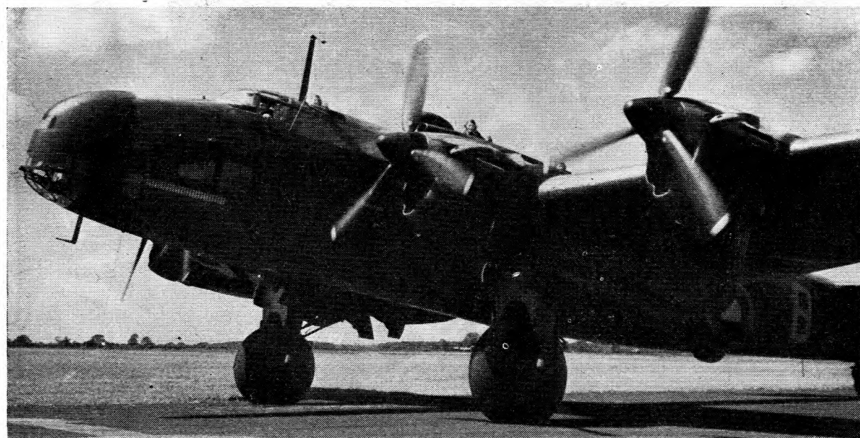
A Halifax II, series I, with a streamlined and cleaned-up nose, having its engines run over after returning from a raid.
