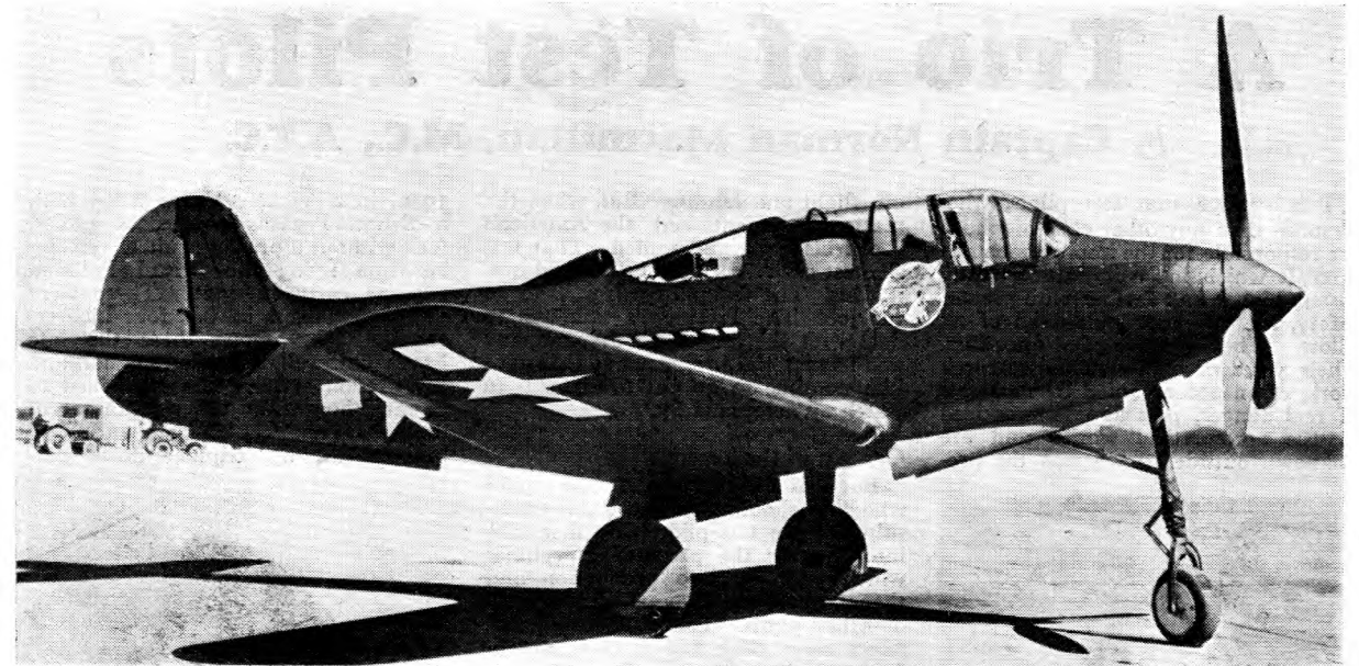
This Bell Airacobra has been converted into a trainer for fighter pilots likely to fly tricycle undercarriage aircraft. The cockpit cover has been extended and nose armament removed.
