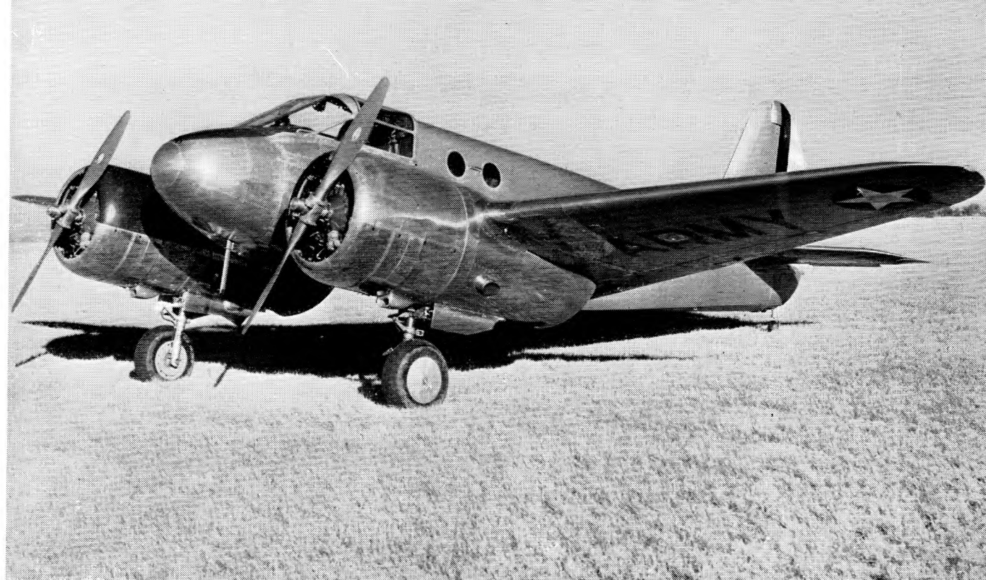
The Beech AT-10 (above) is the first all-wood advanced trainer to be used by the U.S.A.A.F. After tuition on the AT-10 the pupil will pass on to operational types, such as the B-17G Fortress below.
