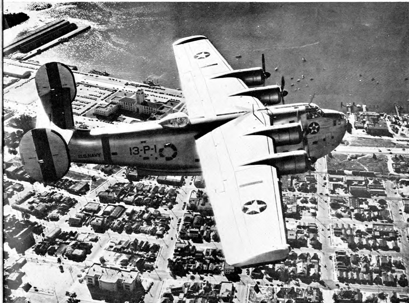
Evening outing. A 9th Air Force Marauder makes a striking picture as she heads for home after a bombing mission. Below is an overhead view of one of the U.S.N.'s Coronados flying over the sun-dried scenery of San Diego, California. Wing span, 115 ft.; top speed, 220; weight, loaded 30 tons.
