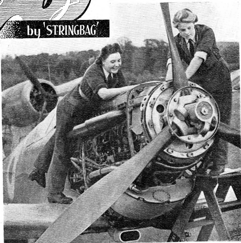
Two WAAFS work on the Merlin engine of a Spitfire as part of their fitters' (engines) course with Technical Training Command.
