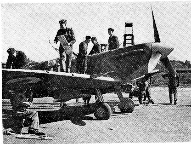
Ground staff rearming a Spitfire just returned from a fighter sweep. Immediately after landing, the machine is examined for damage, serviced and made ready again for instant take-off.
