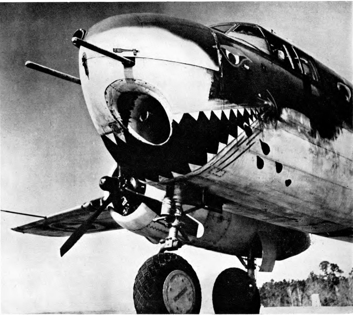
The Mitchell seen in the top picture is one of the older version extensively used in European operations. The gaping sharks' teeth belong to a South Pacific Mitchell, one of the many dishing it out to the Japs, armed with a handy 75-mm. cannon. These aircraft have been known to sink Jap ships with one burst.
