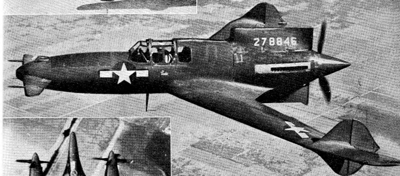
Top left and above is the Curtiss XP-55 Ascender, single-seater pusher pursuit. Elevators are in the extreme tip of the nose, and rudders near the wing tips. On the left is the twin-engine long-range interceptor, McDonnell XP-67. The Fisher XP-75 below started out as a composite of several other kinds of aircraft and this design emerged. A 3,000-h.p. Allison located behind the pilot drives contra-rotating airscrews. At the foot of the page is the Vultee XP-54, twin-boomed pusher. No performance details are available.
