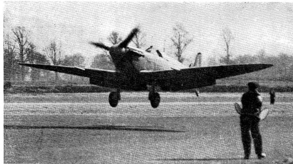
Seafire doing a dummy deck landing on a Nava' fighter station. The batsman has just indicated "cut" by crossing the bats. Notice the nose-up 3-point position of the aircraft.
