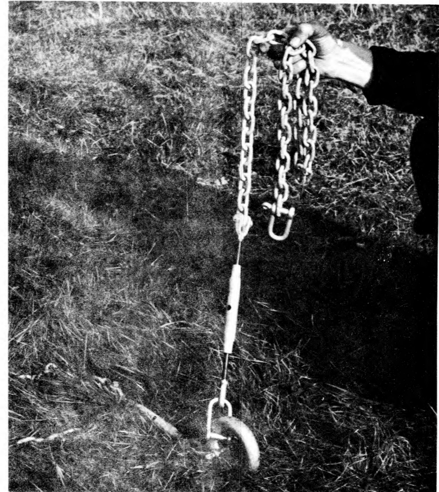
FIG . 11 . CONNECTIONS TO GROUND ANCHOR
