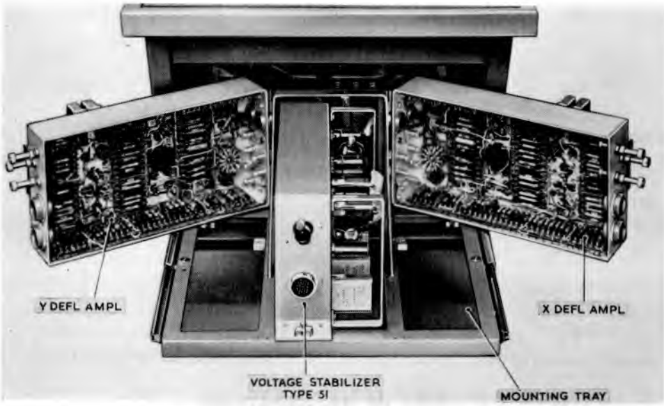
Fig. 1. Lower half of console Type 64 (Mounting tray drawn forward, and deflection amplifiers swung out)
