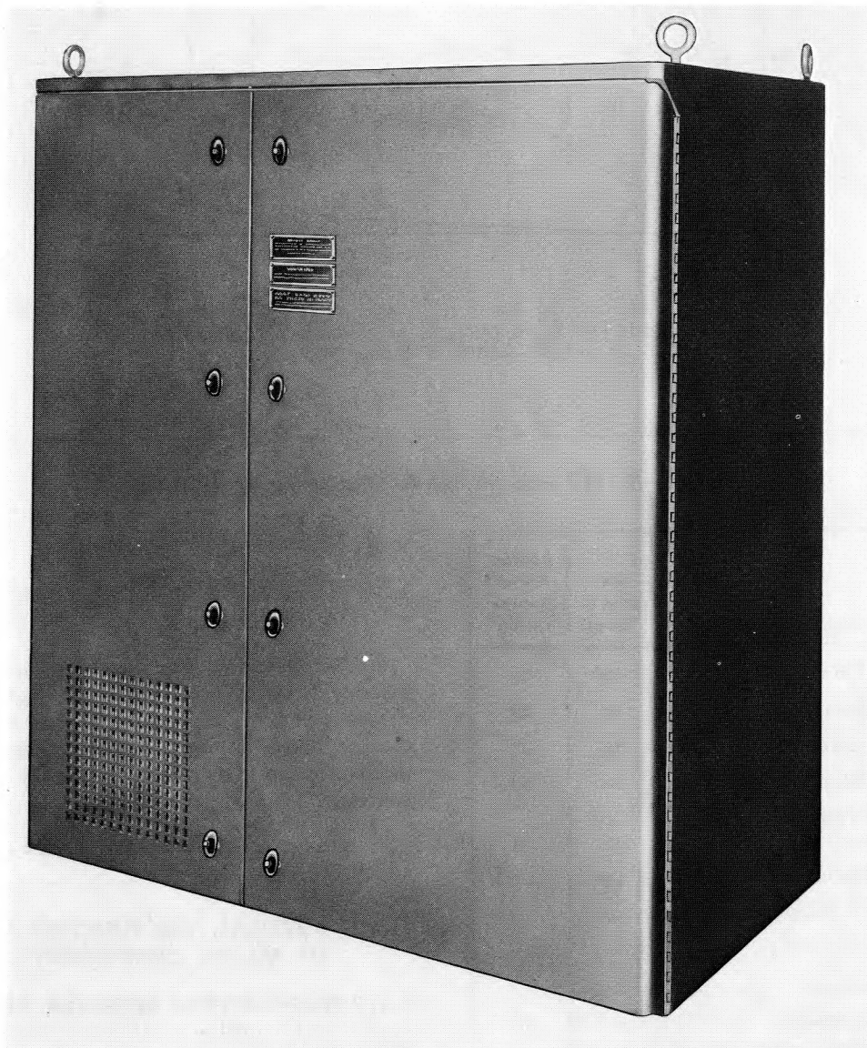
Figure 1-11. R-f Assembly; Radar Set Group OA-357/FPS-6
