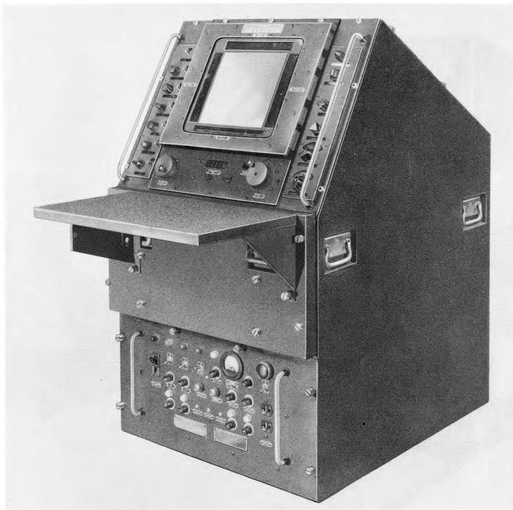
Figure 1-31. RHI Assembly; Radar Set Group OA-270/FPS-6
