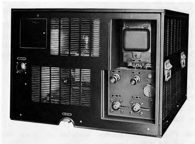
Figure 1-18. Heat Exchanger for Magnetron; Cooler, Liquid, Electron Tube HD-188/FPS-6
