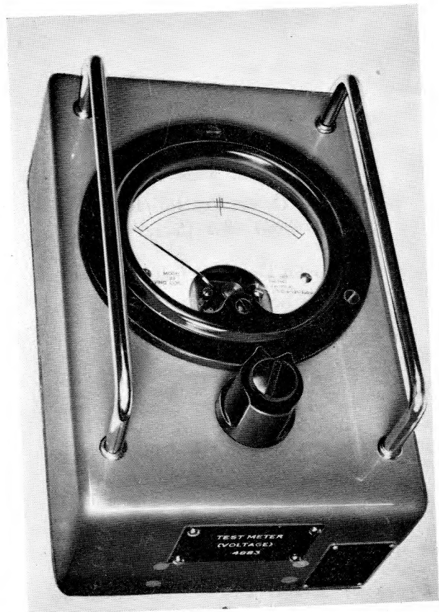
Fig. 4. Test meter (voltage) 4883 : exterior view
