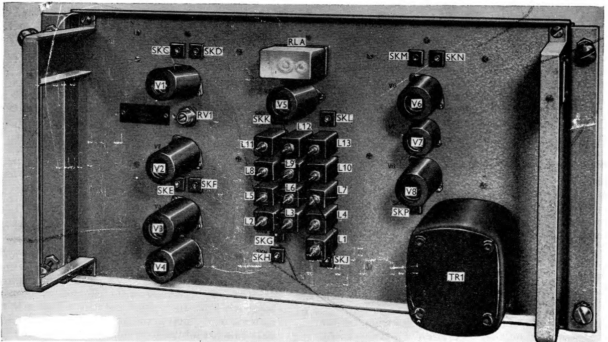
Fig. 1. Switch electronic (clutter) M1 : front view
