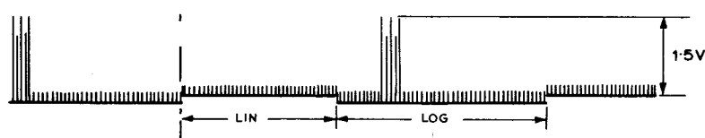
V2 GRID INPUT WAVEFORM (SWITCHING PLUS VIDEO) WAVEFORM DRAWN IN UNBALANCED STATE. ADJUST RV1 FOR BALANCE
