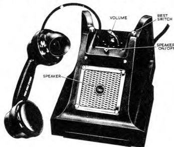
Extension control unit Type 8105A (10L/16540) FGRI 23081/1D, Transmitter-receiver with control unit and extension control
