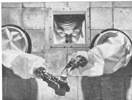
Remote handling of radio-active Gold 198 at Amersham. Protected by lead bricks, the operator views his actions through a lead glass window
