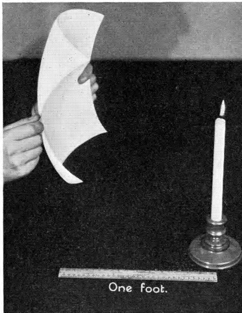
Fig. 2.—THE FOOT CANDLE AND THE LUMEN.
