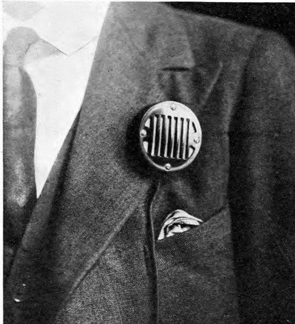
THE IGRANIC BUTTONHOLE MICROPHONE AS WORN FIXED IN THE LAPEL OF THE JACKET.
