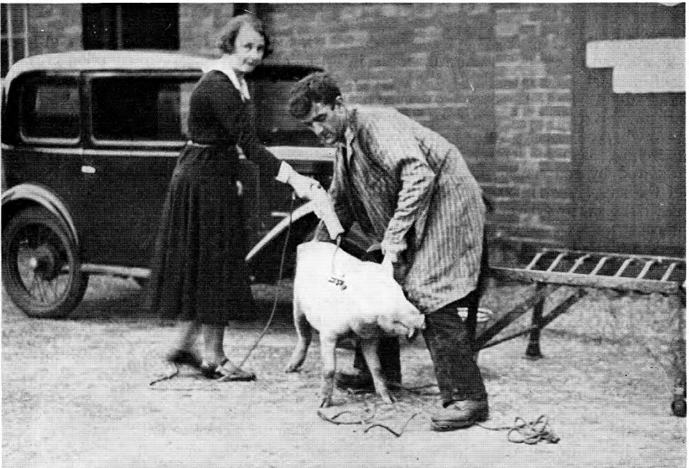
USING THE "ANESTYGUN" FROM A CAR BY MEANS OF A ROTARY CONVERTER WORKING FROM THE BATTERY.
