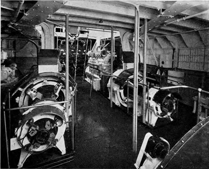
Fig. 1. —AN INTERESTING EXAMPLE OF ELECTRIC SHIP PROPULSION—THE FIRST BRITISH DIESEL-ELECTRIC TUG.
