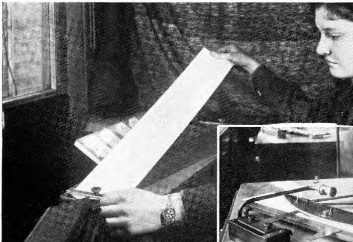
Fig. 5.—FINISHED CALIBRATED CHART WHICH IS MARKED WITH INSTRUMENT NO., DATE AND TEMPERATURE, OPERATOR'S SIGNATURE.
