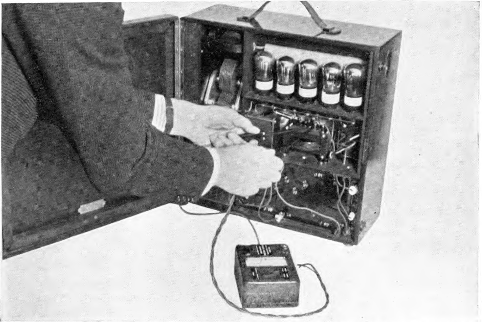
Fig. 6.—USING THE CIRCUIT-TESTING OHMMETER FOR TESTING THE WINDINGS OF A TRANSFORMER IN A RADIO SET.
