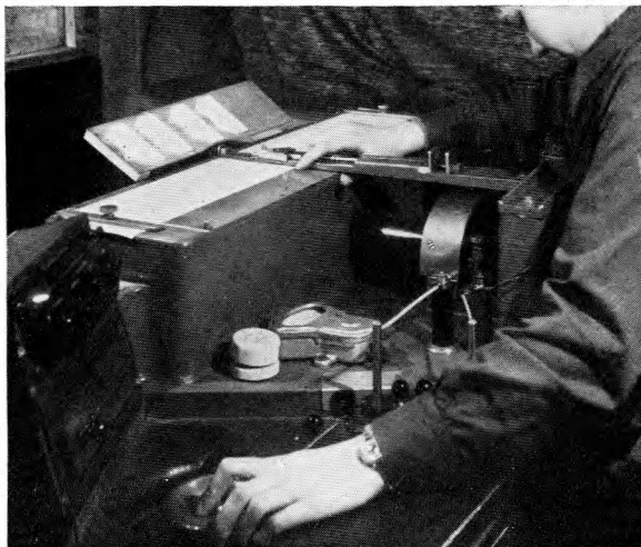
Fig. 3.—CALIBRATOR CHART HALF FINISHED. OPERATOR CHECKING LINE ON DIAL OF INSTRUMENT THROUGH EYEPIECE, AND ADJUSTING KNOWN RESISTANCE WITH LEFT HAND.
