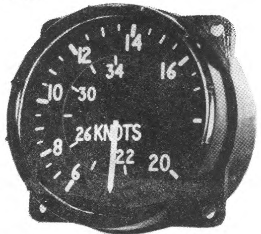
Fig 3 A Typical Simple ASI
