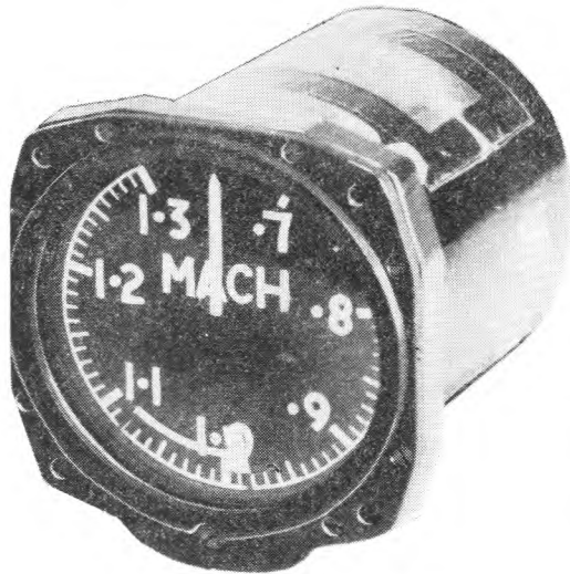
Fig 1 A Typical Machmeter
