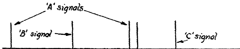
FIG. 2. "B" and "C" Slave Signals on Time Base.
