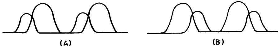
Figure 6-8. Overall System Delay Measurement Waveforms
