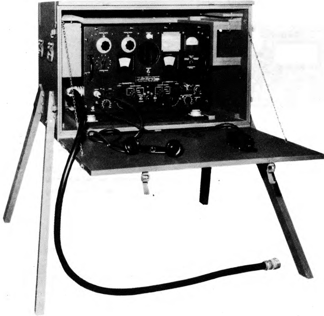
FIGURE 1531. Radio Receiver and Transmitter (Jefferson 350A)
