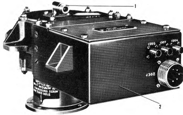
Figure 33. Special Assembly, Direction Finder Group
