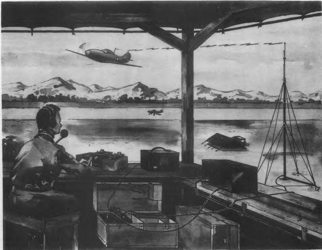
Radio Set SCR-624 provides an easily assembled short range ground - to air command communications facility for use at newly established landing strips and on captured enemy air fields.
