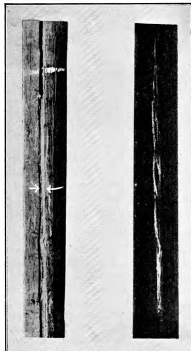
FIG. 6.—SPLINTERING OF TELEGRAPH POLE (LEFT) BY LIGHTNING AND (RIGHT) MODEL POLE SPLINTERED IN THE LABORATORY BY IMPULSE GENERATOR.
