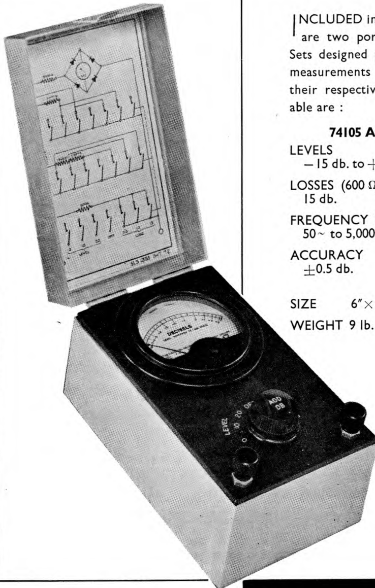
74105 B Transmission Measuring Set
