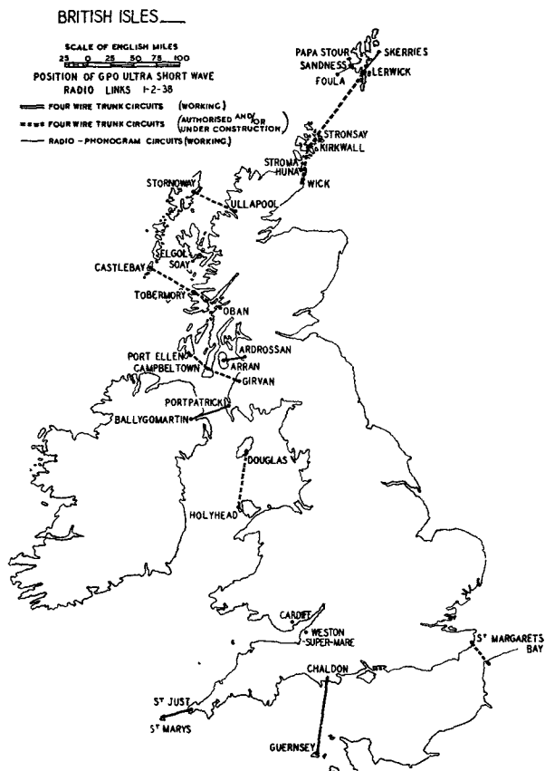
FIG. 13 —U.S.W. RADIO LINKS INSTALLED IN THE BRITISH ISLES.
