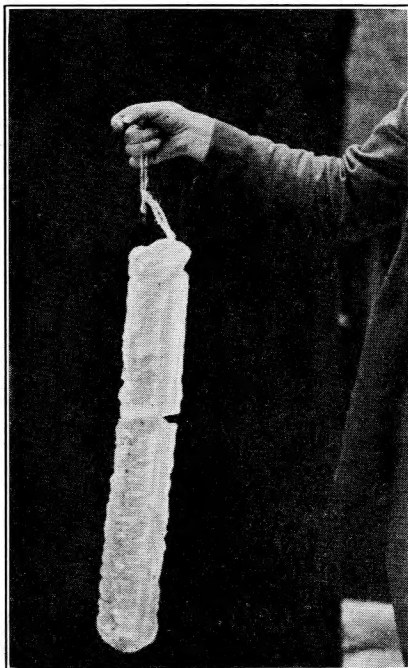
FIG. 1.—A TYPICAL ICE-COATED WIRE, WORCESTER.
