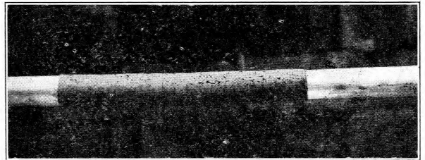
FIG. 2.—CABLE TAPED FOR 10 IN.
