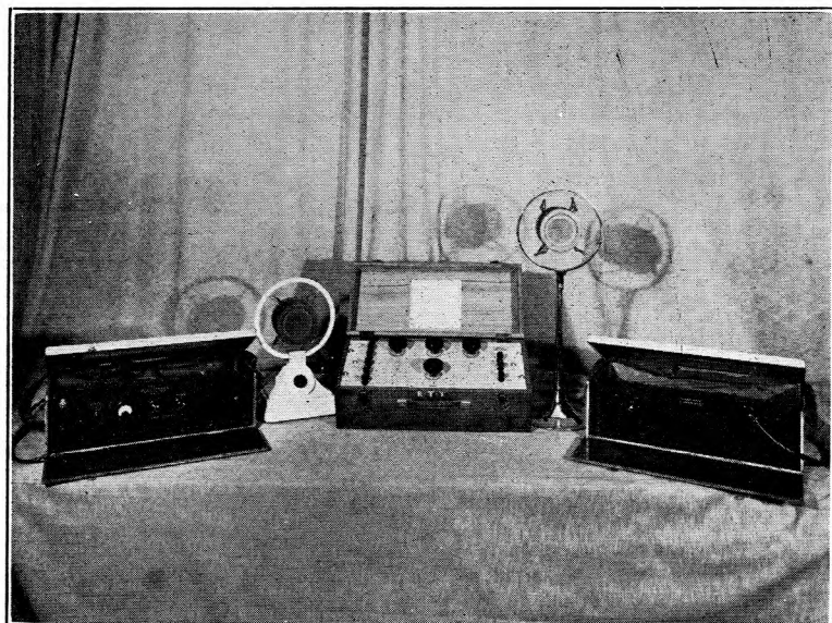
FIG. 1.—MOVING COIL MICROPHONES IN STANDS, MICROPHONE AMPLIFIER AND POWER-PACK, AND MIXING BOX.
