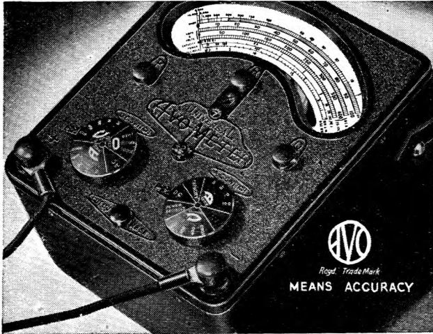
50-range Model 7 Universal AvoMeter
