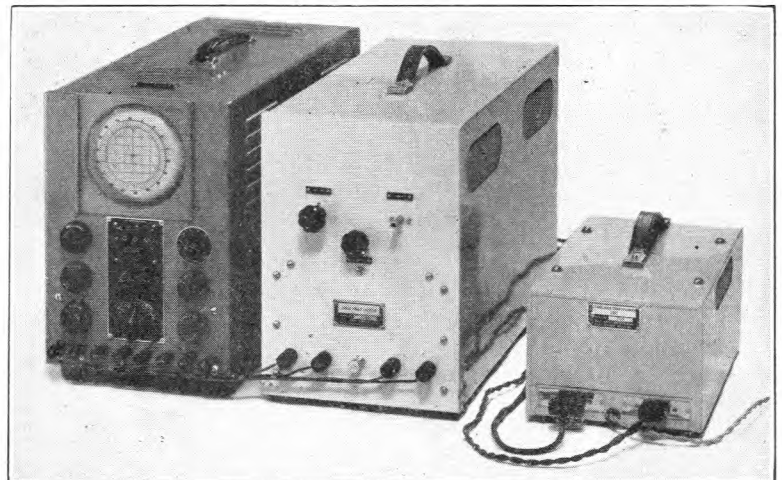
FIG. 2.—CABLE FAULT LOCATOR.
