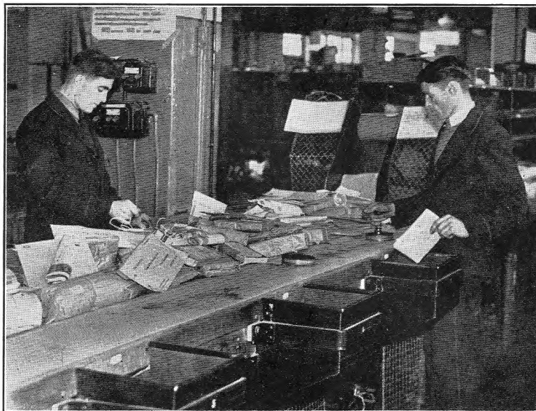
FIG. 1.—HAND-STAMPING TABLE WITH CHUTES.
