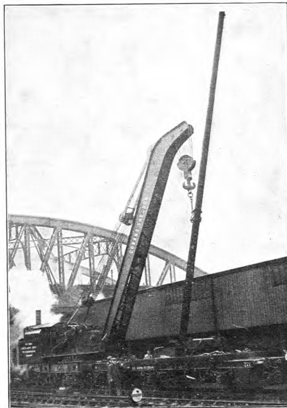
BRITISH RAILWAYS' 45-TON STEAM CRANE RECOVERING 70 FT. POLE AT PETERBOROUGH.
