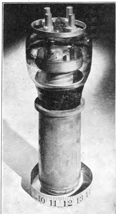
FIG. 3.—SINGLE-ENDED 20-KW WATER-COOLED TRIODE WITH THORIATED-TUNGSTEN FILAMENT.
