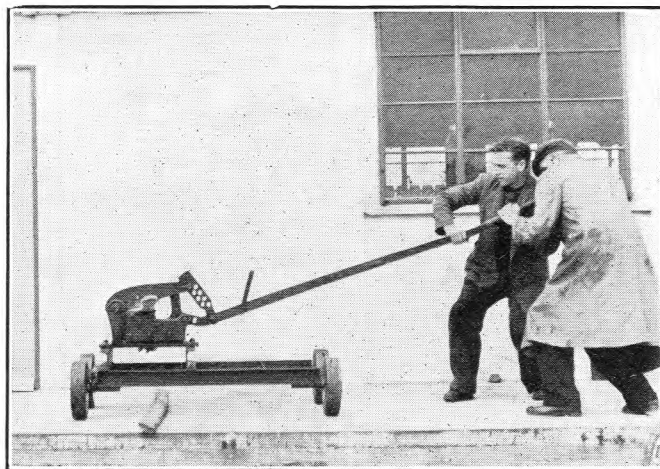
CUTTING CABLE WITH THE GUILLOTINE.
