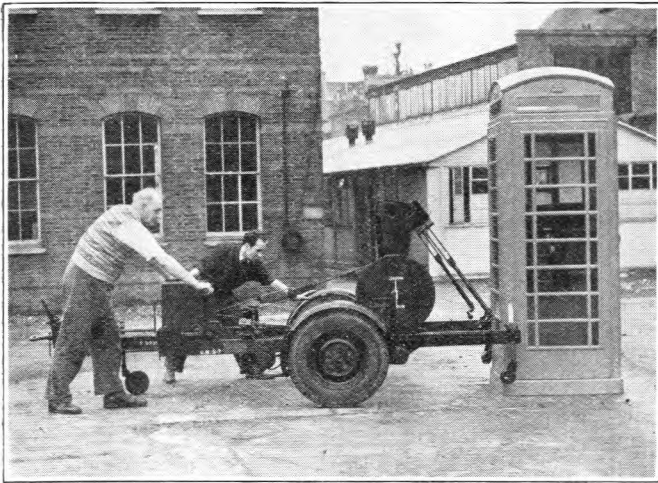
FIG. 1.—PLACING TRAILER AROUND KIOSK.
