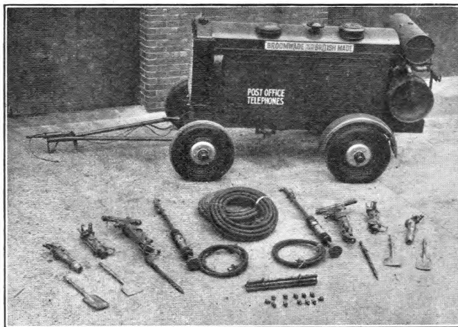
FIG. 4.—TWO-TOOL TRAILER AIR-COMPRESSOR AND TOOL EQUIPMENT.
