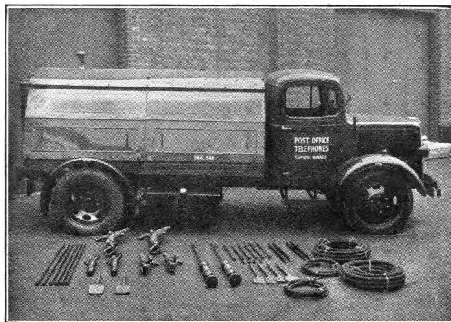
FIG. 1.—SELF-MOBILE AIR-COMPRESSOR AND TOOL EQUIPMENT.
