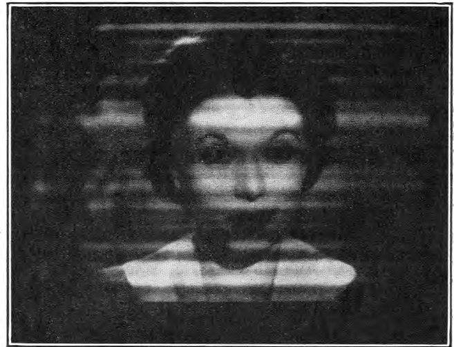
FIG. 4.—PICTURE WITH ADDED AUDIO SIGNAL, ILLUSTRATING "SOUND BREAK-IN."
