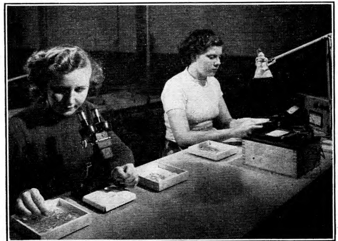
FIG. 7.—FINAL INSPECTION OF IA THERMISTORS.
